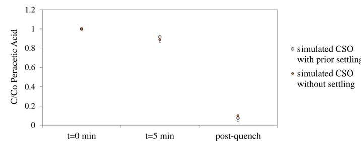
Figure 1 PAA concentration remaining (C) compared to initial PAA concentration ( $C_0$ ) initially (t=0min), after during 5 minutes of disinfection with 5 mg/L nominal PAA concentration (t=5min), and after quenching the disinfection reaction (post-quench).<sup>7</sup>
