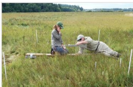
K. Turner (USGS WERC) and G. Guntenspergen (USGS PWRC) reading SET, Nisqually Reference Marsh.
